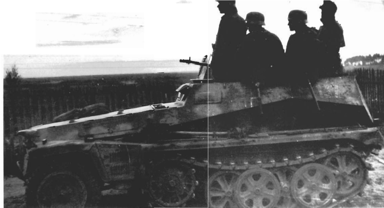
Above: A light Schützenpanzerwagen (Sd.Kfz.250/1), below a medium type (Sd.Kfz.251/1). The upper one could transport six men, the lower one twelve — counting the driver and commander. (2 x BA)
