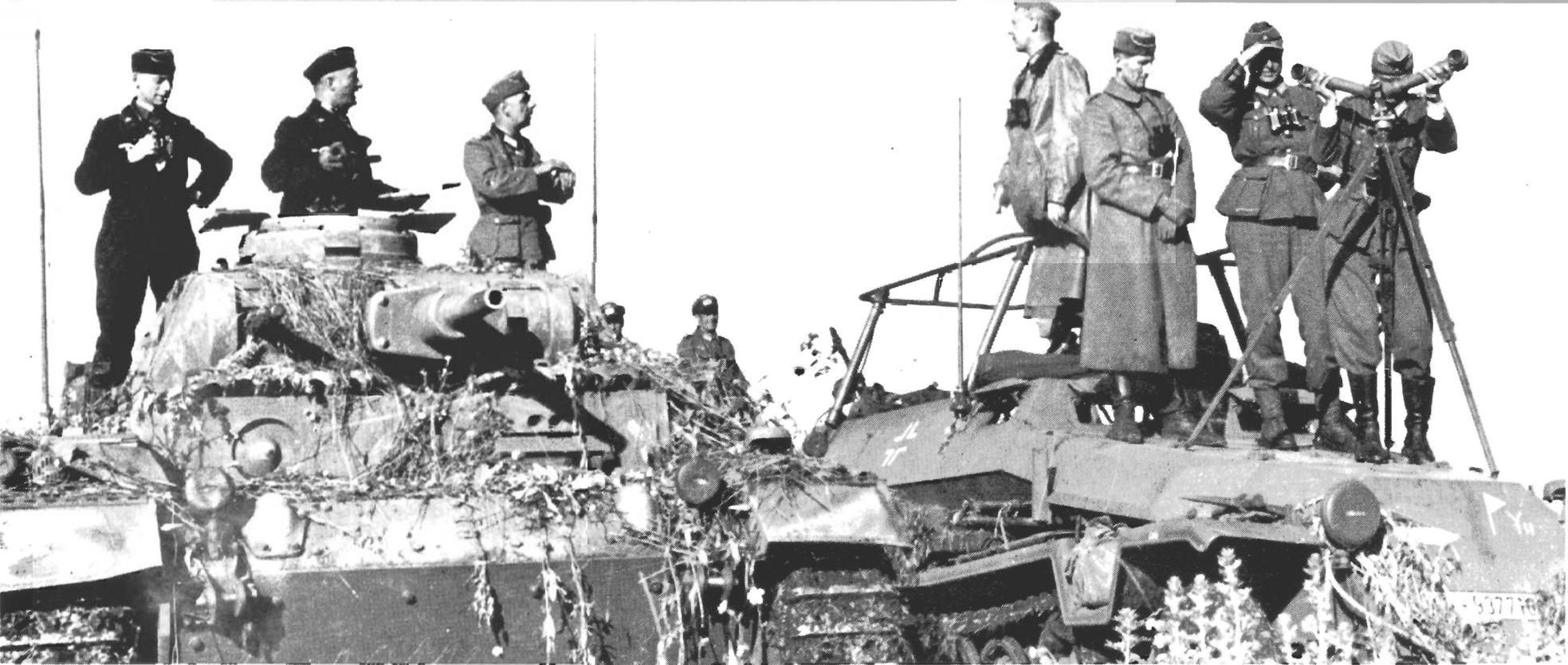
Above: Beside a Command Panzer III (two antennas) stands a SPW, Sd.Kfz.251/3 or /6, of a rifle battalion of the 9th Panzer Division (note tactical and division emblems on the nose of the SPW). Here a Panzer unit commander is talking with the commander of a rifle battalion.
